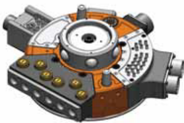
3 Model for exchanging hands or jigs on actuated servo motors.
