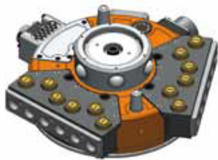
2 Model for exchanging jig hands for material handling.
