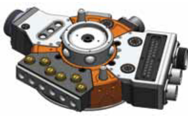
5 Model for exchanging spot welding guns and for handling hands or jigs.
